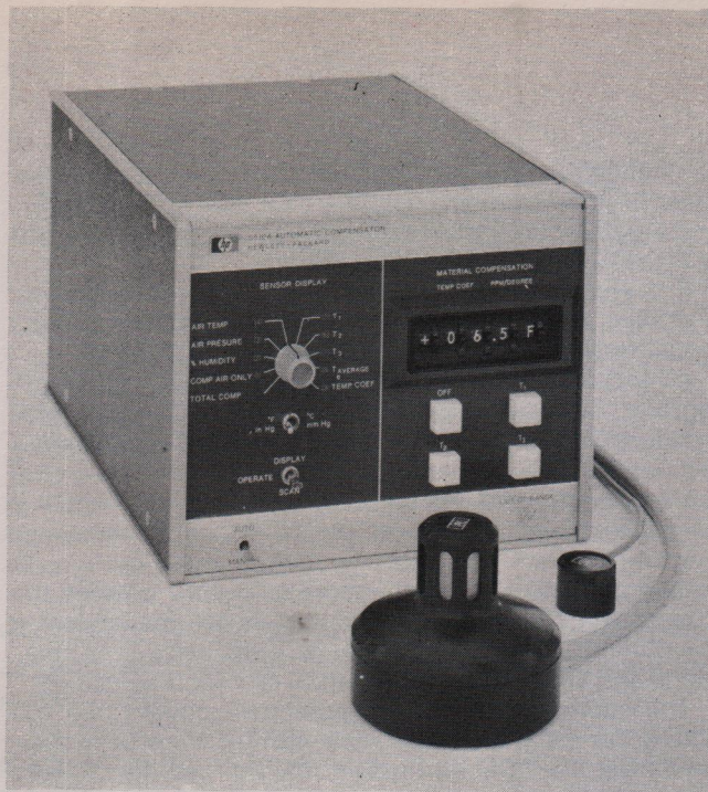
2. Compensation. Errors produced by thermal and other factors are corrected by 5510A automatic compensator. The probes have magnetic bases for easy attachment near the measurement path.
